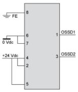
With External Device Monitoring (EDM) feedback loop
