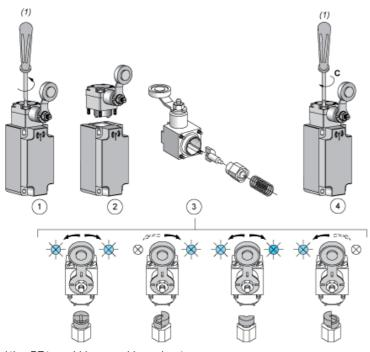
$\begin{array}{lll} \text{(1)} & \text{PZ1, pozidriv screwdriver, size 1} \\ \text{C:} & 1 \text{ Nm ($\pm$ 20 %) / 8.85 lb-in ($\pm$ 20 %)} \\ \end{array}$
