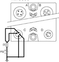
(3) External fuse, Type T slow-blow, 8 A max., 250 V PS2 External isolated I/O power supply, 24 Vdc
