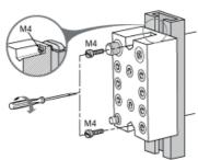
NOTE: Maximum torque to fasten the required M4 screws is 0.6 N.m (5.3 lbf-in).
