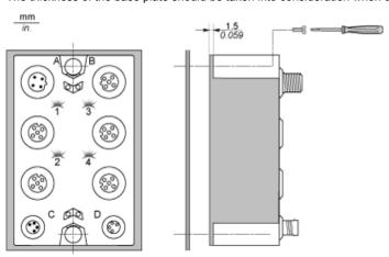
NOTE: Maximum torque to fasten the required M4 screws is 0.6 N.m (5.3 lbf-in).
