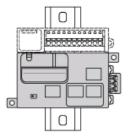
NOTE: Expansion modules must be mounted above the controller.
