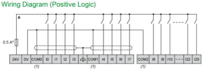
(\*): Type T fuse(1): The COM0, COM1 and COM2 terminals are not connected internally.
