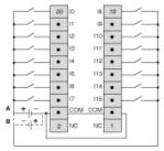
A Sink wiring (positive logic)
