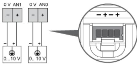
The (-) poles are connected internally.
