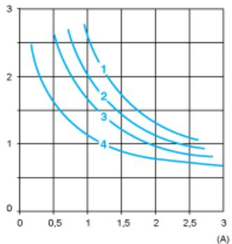
AC-14 Control of weak electromagnetic loads of electromagnets  $\leq 72$  VA (make:  $\cos \phi = 0.3$ , break:  $\cos \phi = 0.3$ )
