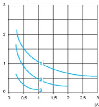
DC-13 Control of electromagnets ( $L/R \leq 2 \times (U_e \times I_e)$  in ms, with  $U_e$ : rated operating voltage and  $I_e$ : rated operating current)
