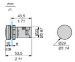
e Support panel thickness: 1 to 6 mm/0.4 to 0.24 in. (metal), 2 to 6 mm/0.8 to 0.24 in. (plastic).
