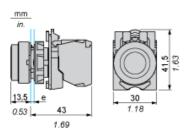
clamping thickness: 1 to 6 mm / 0.04 to 0.24 in. e:
