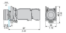
e: clamping thickness: 1 to 6 mm / 0.04 to 0.24 in.
