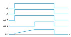
Us: Power supply voltage Uc: Control supply voltage LED Green LED
