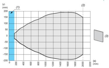
(X): Target distance (Y): Detection limit
