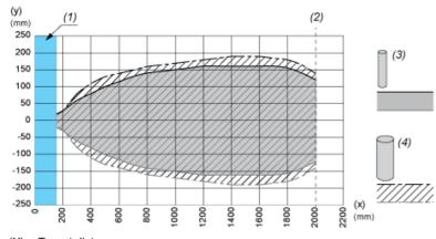
(X): Target distance (Y): Detection limit
