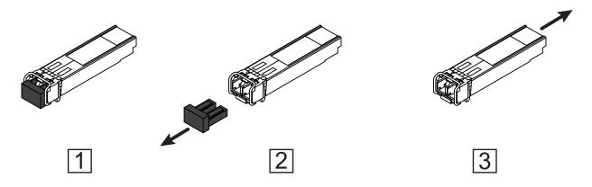
Figure 10: Installing SFP transceivers: Installation sequence
