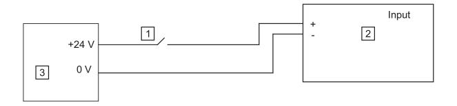
Figure 16: Connection of a sensor with separate power supply
