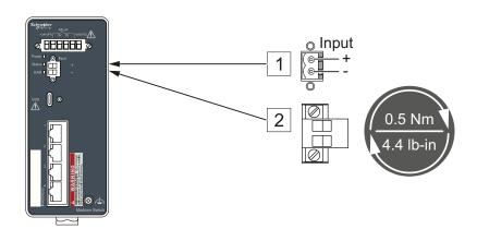
Figure 7: (1) Connection on the device, (2) terminal block mounted on the device (front view), tightening torque.
