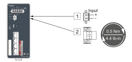
Figure 14: (1) Connection on the device, (2) terminal block mounted on the device (front view), tightening torque.
