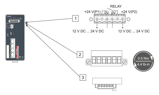
Figure 11: (1) DC voltage connection on the device, (2) terminal block mounted on the device (front view), tightening torque, (3) terminal block mounted on the device (view from above).
