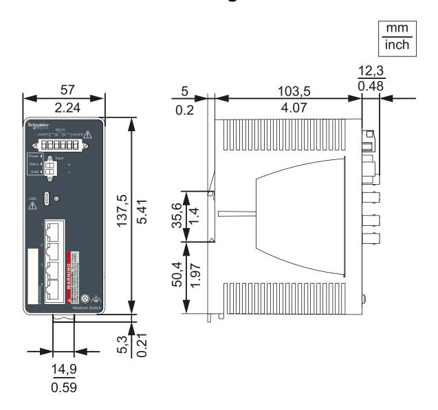
Figure 19: Device variants with 4 ... 6 ports without PoE
