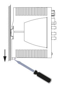
Figure 18: Removal from the DIN rail
