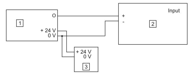
Figure 15: Connection of a sensor with separate power supply
