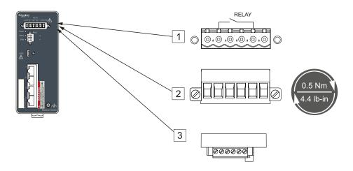
Figure 13: (1) Connection on the device, (2) terminal block mounted on the device (front view), tightening torque, (3) terminal block mounted on the device (view from above).
