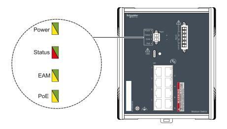
Figure 1: LED display elements for device status
