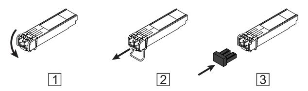
Figure 17: De-installing SFP transceivers: De-installation sequence
