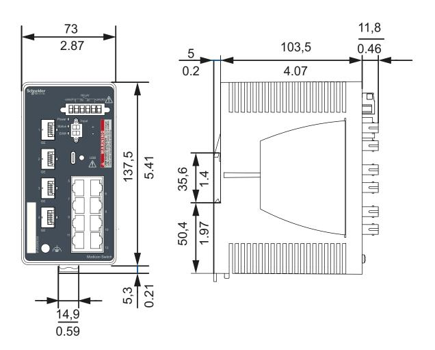
Figure 20: Device variants with 8 ... 12 ports without PoE
