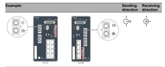
Table 5: Sending and receiving directions for device variants with DSC ports
