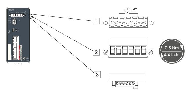
Figure 5: (1) Connection on the device, (2) terminal block mounted on the device (front view), tightening torque, (3) terminal block mounted on the device (view from above).
