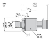
(1) SW24 tightening torque ≤ 25 N.m / 221 lb-in
