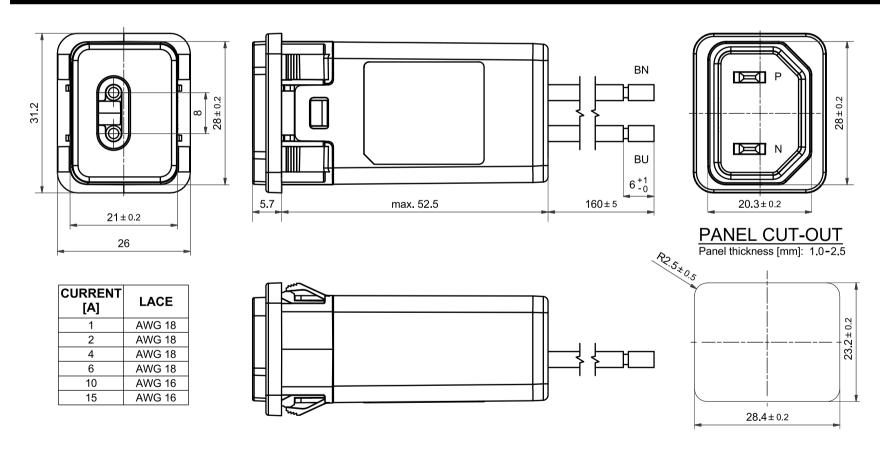
For dimensions [mm] without tolerances: ISO 2768-m / EN22768-m applies
