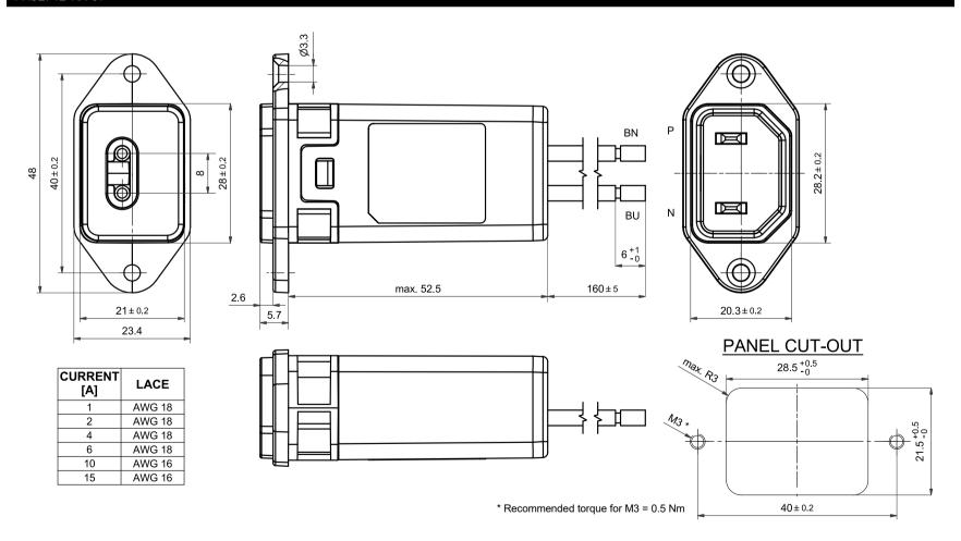
For dimensions [mm] without tolerances: ISO 2768-m / EN22768-m applies
