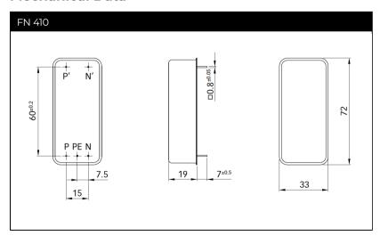
All dimensions in mm; 1 inch = 25.4 mm Tolerances according: ISO 2768-m/EN 22768-m
