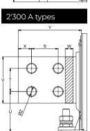
Note: all FN3311 and FN3310 provide unsymmetrical mounting hole patterns to prevent inverse filter installation in the field.
