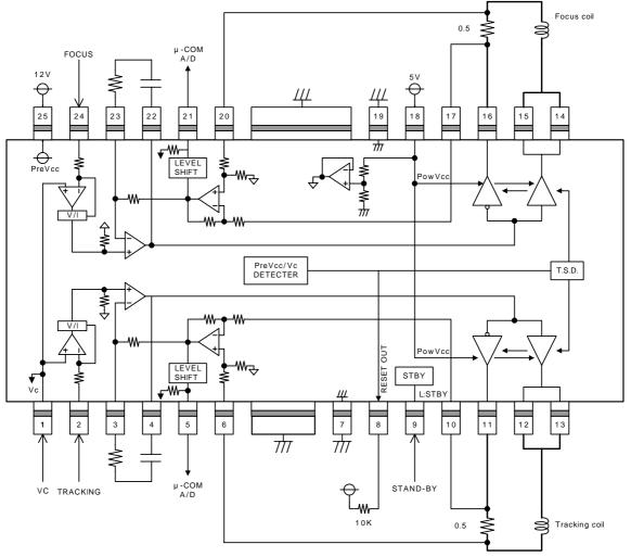
T.S.D: (Thermal shutdown) Resistance unit:  $[\Omega]$
