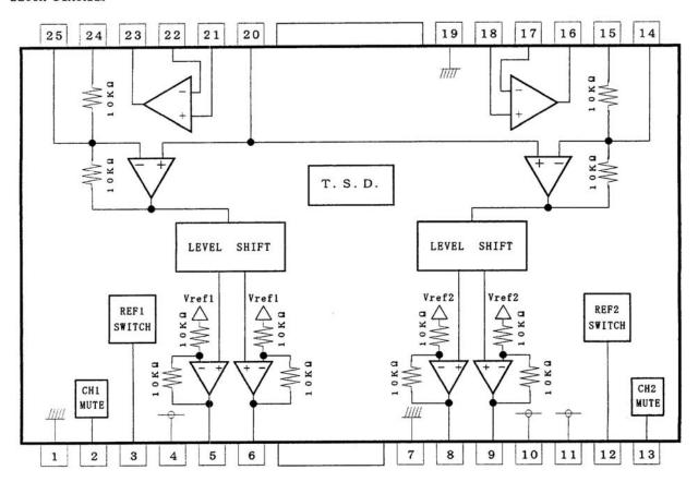
'T.S.D. ; Thermal shut down circuit  $\mbox{Limits for resistance value:}(\Omega) \\ \mbox{Figure 3}$
