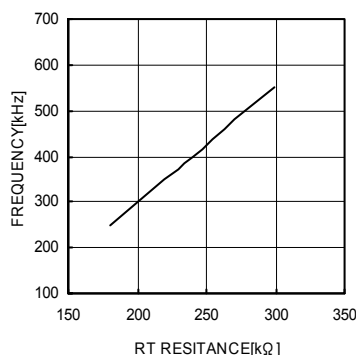
Figure 22. RT resistor vs. oscillation frequency
