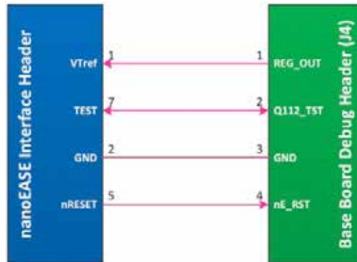
Figure 38: nanoEASE - Base Board Connection Diagram
