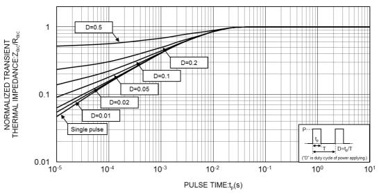
NORMALIZED TRANSIENT THERMAL IMPEDANCE FROM JUNCTION TO CASE (PER DEVICE)
