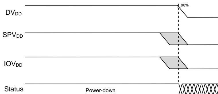
Shut down in order of  $IOV_{DD}$ ,  $SPV_{DD}$ , and  $DV_{DD}$  or  $SPV_{DD}$ ,  $IOV_{DD}$ , and  $DV_{DD}$ .
