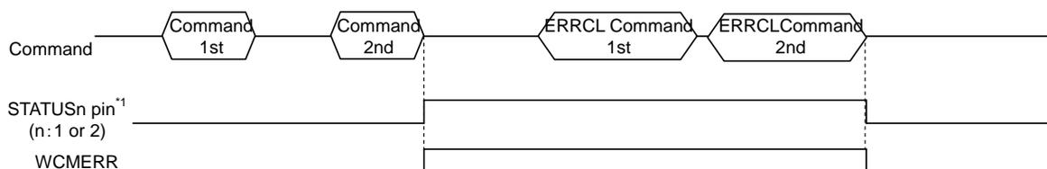
\*1 Misoperation detection and failure detection outputs are selected by OUTSTAT command.
