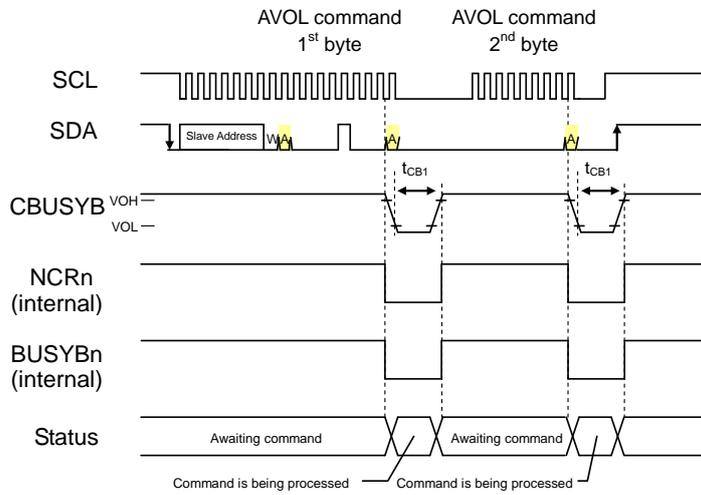
Speaker amplifier volume setting by AVOL commands is valid only when Class AB speaker amplifier is used. When a Class D speaker amplifier is used, the setting value is ignored and +0.0dB is selected.
