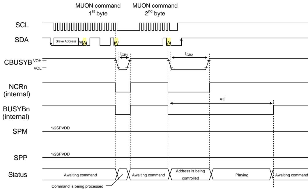
When the first byte of the MUON command is input, the device waits for the input of the second byte after the command processing time ( $t_{CB1}$ ). When the second byte is entered, the silence time is calculated after the command processing time ( $t_{CB2}$ ). When the calculation of the silence duration is completed, the calculated silence is played back, and when the playback is completed, the BUSYB signals of the playback channels become "H" level.
