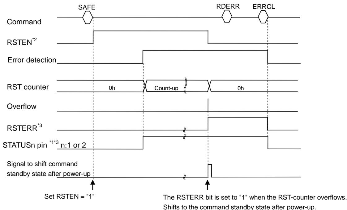
\*1 Misoperation detection and failure detection outputs are selected by OUTSTAT command.
