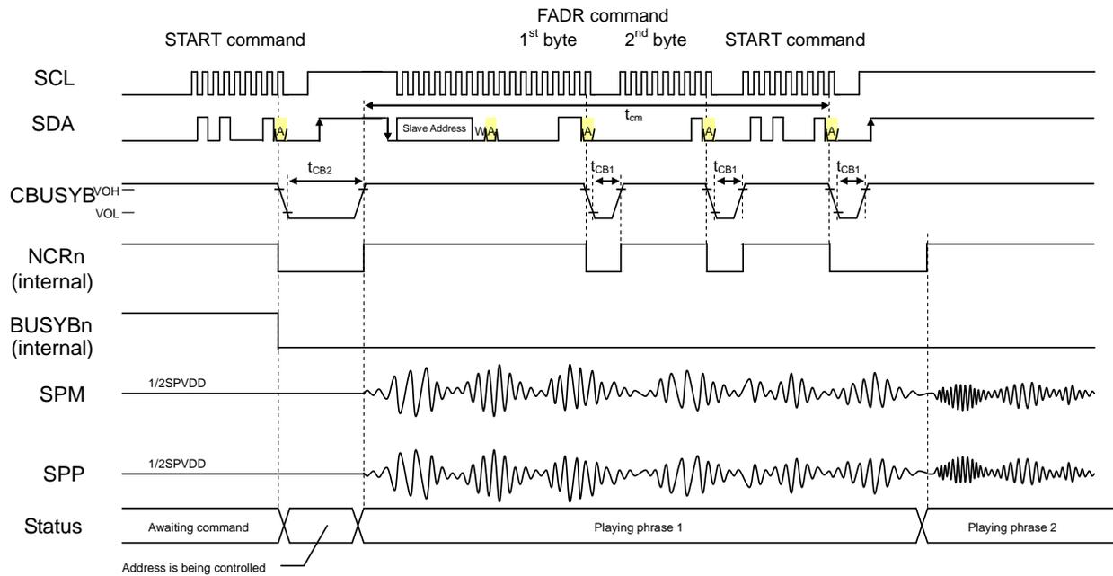
When making continuous playbacks, input the START command for the next phrases within the specified time period ( $t_{cm}$ ) after the NCR of the corresponding channel changes to "H" level, so that the LSI plays back the next phrases without silence sounds after the current phrase playback ends.
