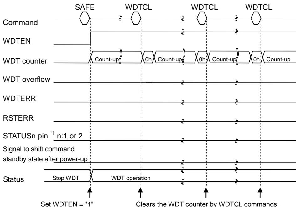
\*1 Misoperation detection and failure detection outputs are selected by OUTSTAT command.
