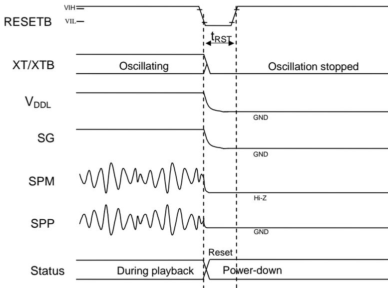
The same timing is applied when a reset is input during command standby.
