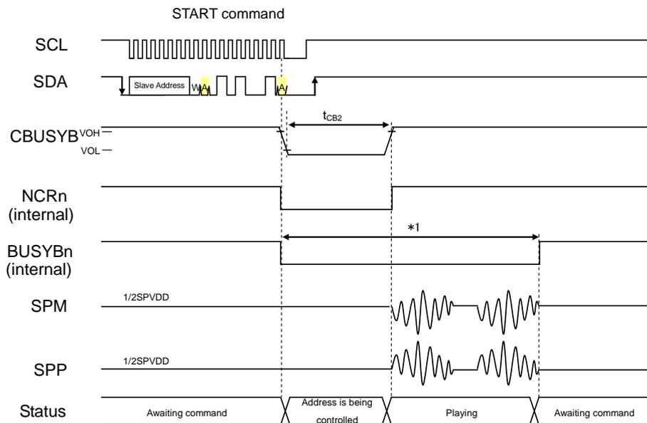
When the START command is input, the address data of the phrase to be played after the command processing time ( $t_{CB2}$ ) is read from the flash memory. When the phrase address data is read, the specified phrase is played back, and when playback is completed, the BUSYB signal of the playback channel becomes "H" level.
