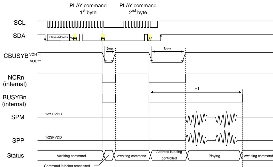
When the first byte of the PLAY command is input, the device waits for the input of the second byte after the command processing time ( $t_{CB1}$ ). When the second byte is entered, the address data of the phrase to be played after the command processing time ( $t_{CB2}$ ) is read from the flash memory.
