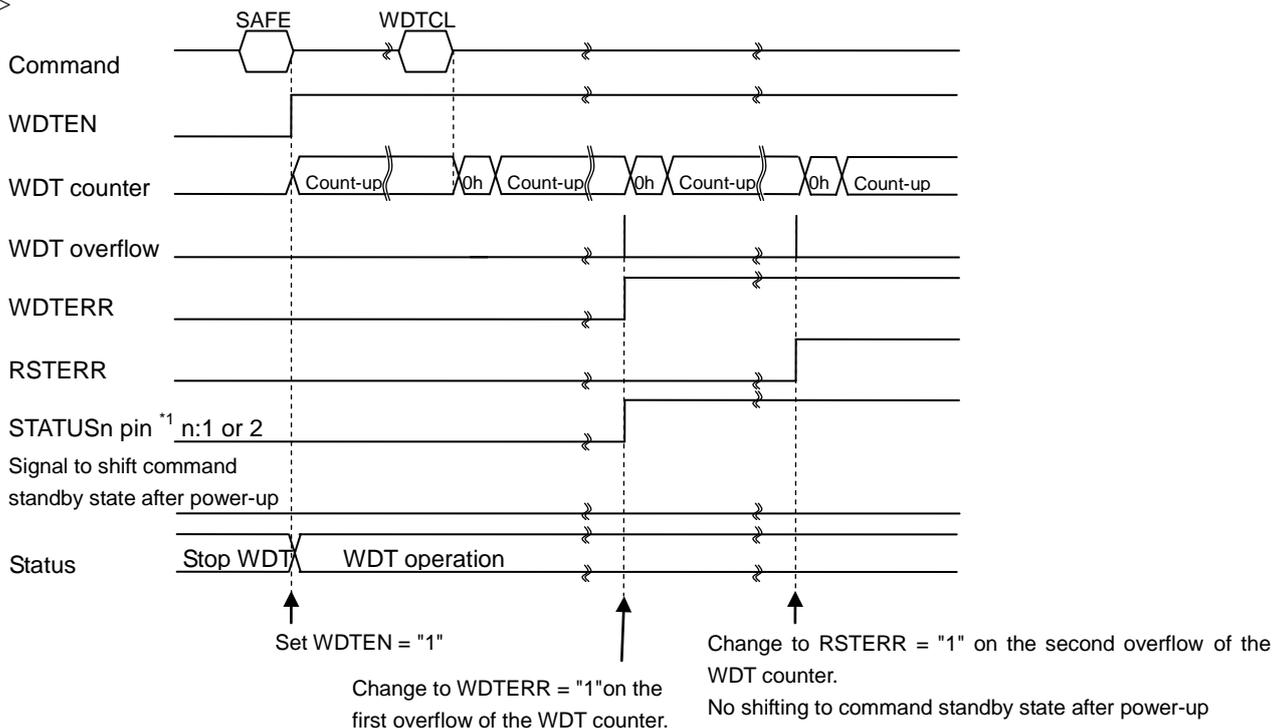
\*1 Misoperation detection and failure detection outputs are selected by OUTSTAT command.
