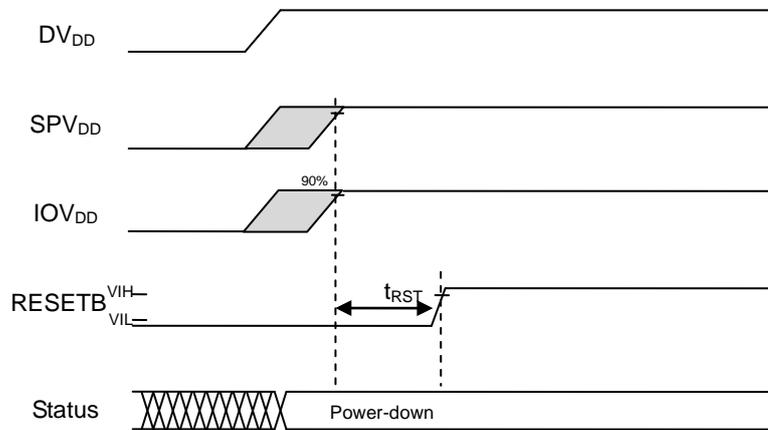
After the power is turned on, the device enters the power-down state.
