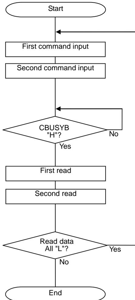
When the OUTSTAT command is used to select the misoperation detection and failure detection outputs and the STATUS1 or STATUS2 pin is "H", if all the read data is "L", the data cannot be read normally. Accordingly, read the data again.
