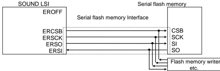
The serial flash memory can be rewritten using the ERCSB, ERSCK, ERSI and ERSO pins that is the serial flash memory interface.
