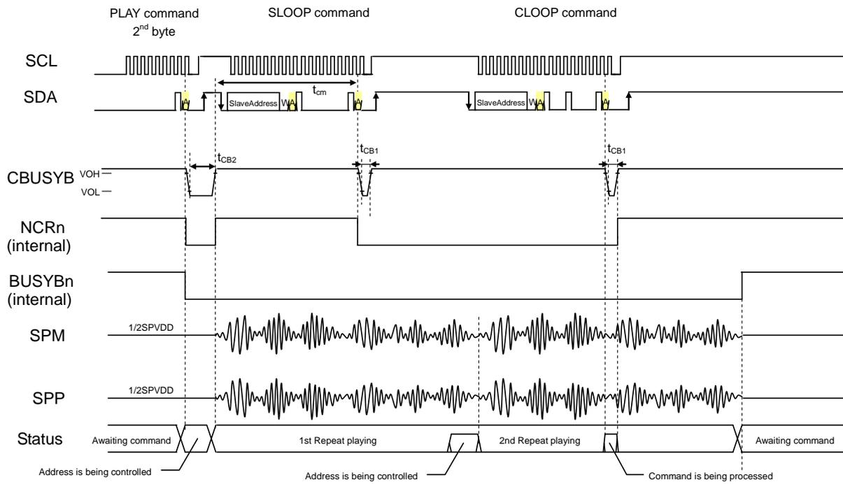
The SLOOP command is valid only during playback. After the PLAY command is input, input the SLOOP command within the specified period ( $t_{cm}$ ) after the NCR of the corresponding channel becomes "H" level. This enables the SLOOP command and repeats playback. While the repeat playback mode is set, the NCR signal is "L" level.
