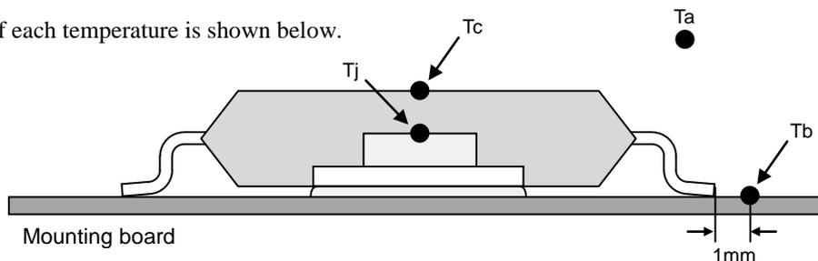
Take measures to dissipate heat on the mounting board so that the maximum junction temperature does not exceed 125°C.
