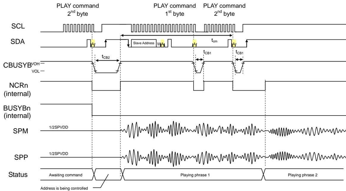
When making continuous playbacks, input the PLAY command for the next phrases within the specified time period ( $t_{cm}$ ) after the NCR of the corresponding channel changes to "H" level, so that the LSI plays back the next phrases without silence sounds after the current phrase playback ends.
