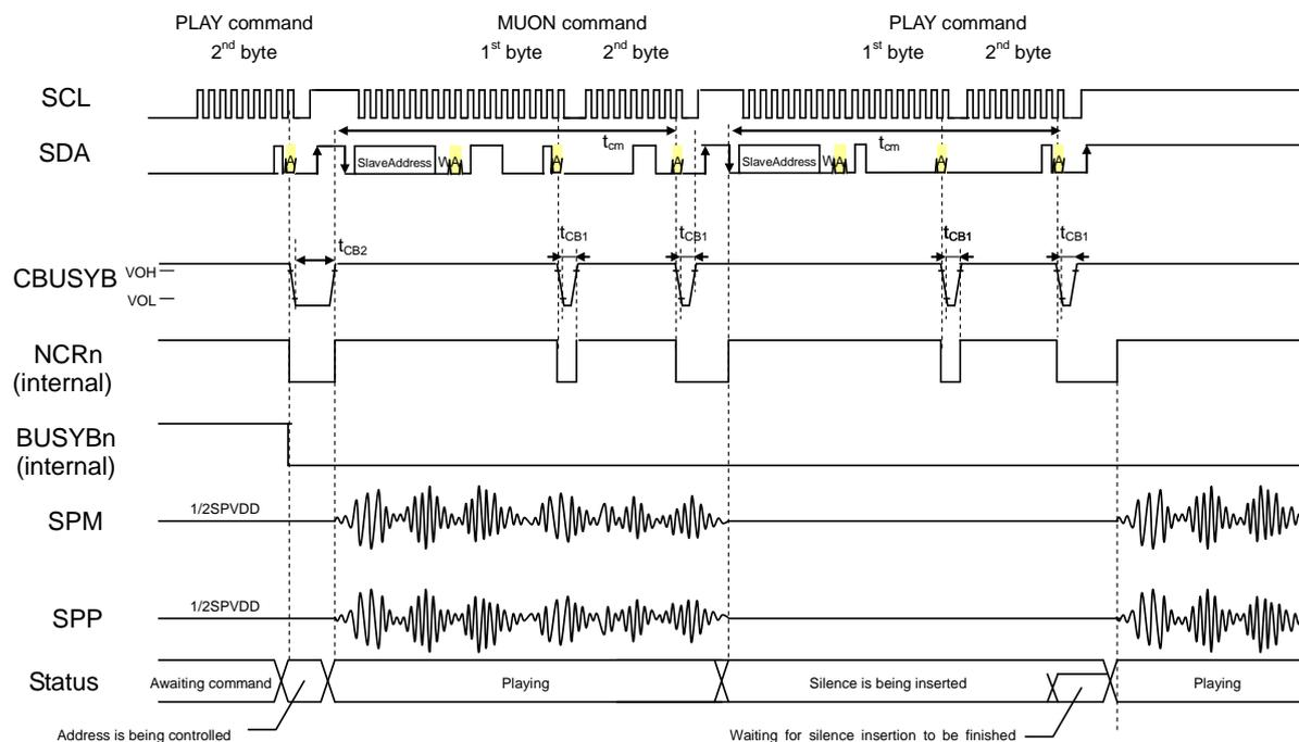
After the PLAY command is input, the CBUSYB signal and NCR signal change to "H" level when the address management of phrase 1 is completed and start playing back. Input the MUON command after the CBUSYB signal changed to "H" level. After the MUON command is received, the LSI is in a state waiting for the end of playback of phrase 1 and the NCR signal remains "L" level until the end of playback.
