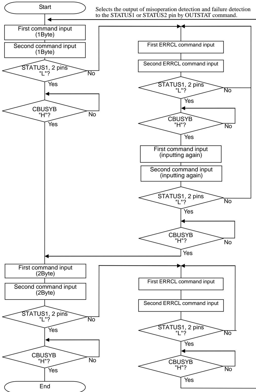
● 3-byte command input flow in two-times input mode
