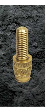
The body of this threaded stud is specifically modeled after our H Series Insert. Its key feature is the tapered design, which allows for easy insertion into tapered molded or drilled holes. They may be installed using the thermal or ultrasonic method or can be molded in place.
