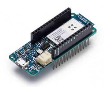
Arduino MKR1000 has been designed to offer a practical and cost effective solution for makers seeking to add Wi-Fi connectivity to their projects with minimal previous experience in networking. It is based on the Atmel ATSAMW25 SoC (System on Chip), that is part of the SmartConnect family of Atmel Wireless devices, specifically designed for IoT projects and devices.
