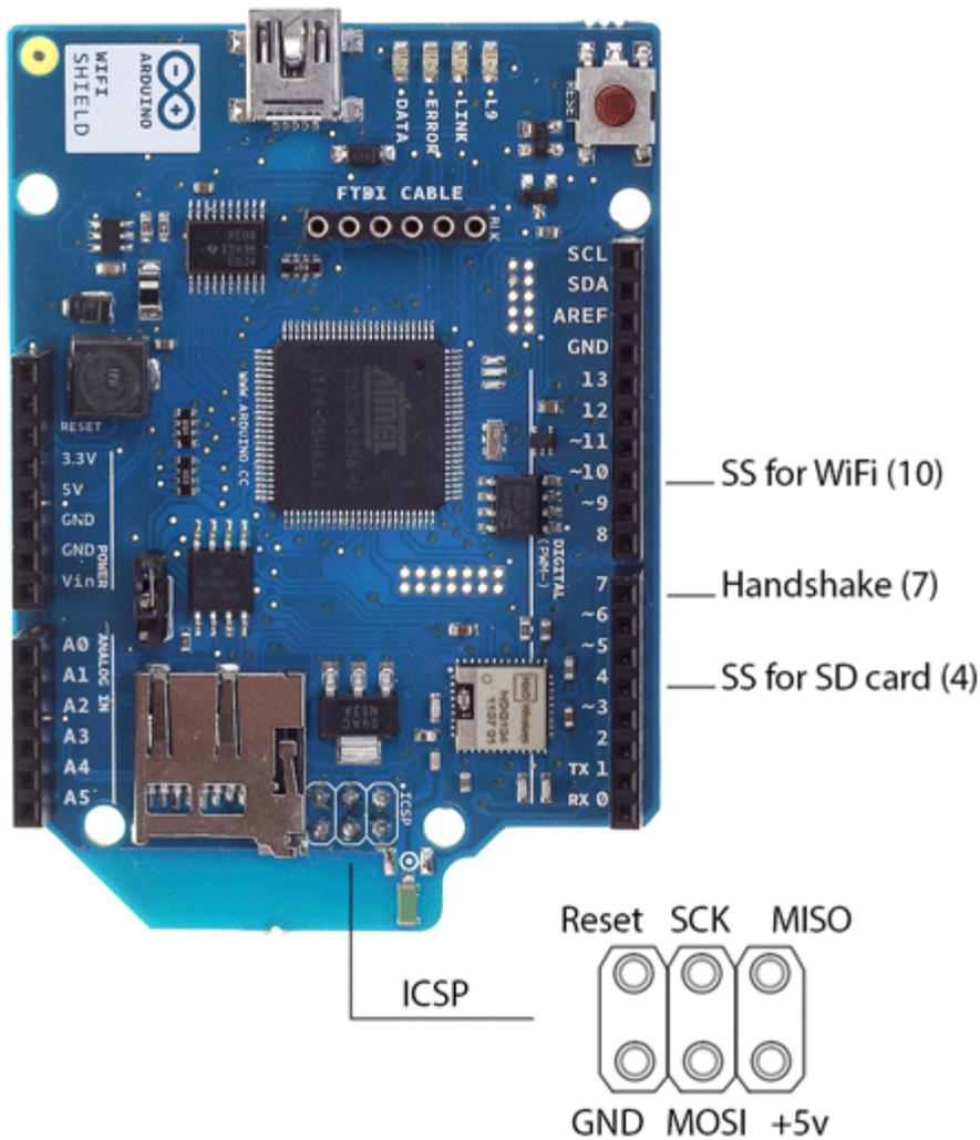
To use the shield, mount it on top of an Arduino board (e.g. the Uno). To upload sketches to the board, connect it to your computer with a USB cable as you normally would. Once the sketch has been uploaded, you can disconnect the board from your computer and power it with an external power supply.
