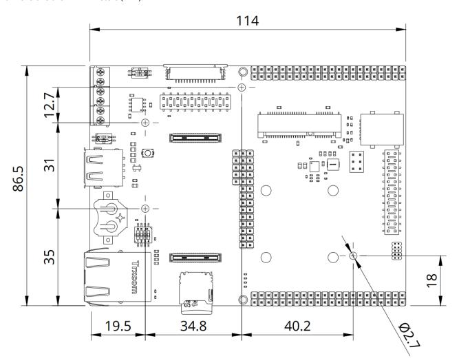
The carrier has four 2.7 mm drilled mounting holes for mechanical fixing.
