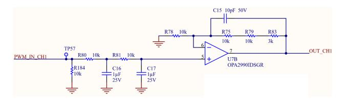
At each input of each channel a PWM from Portenta is provided filtered by a double low pass filter, obtaining a DC output with a small AC ripple. The signal is then fed to the channel non inverting amplifier which amplifies it by 3.3.
