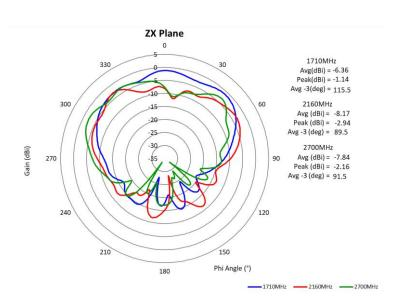
1710MHz 330 on Avg(dBi) = -6.13Peak(dBi) = -0.96 Avg -3(deg) = 98.5 2160MHz 300 Avg (dBi) = -9.52 Peak (dBi) = -3.86 Avg -3 (deg) = 72.5 -25 2700MHz Gain (dBi) Avg (dBi) = -8.63 270 90 Peak (dBi) = -1.74 Avg -3 (deg) = 36.5 240 120 210 150 Phi Angle (°) 180 -1710MHz -2160MHz -2700MHz
