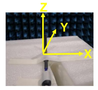
Antenna is a monopole antenna. All data in this document is tested without any additional ground plane. Antenna in free space.
