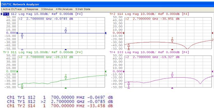
Ch1 Tr1 S12 >2 2.7000000 GHz -0.0785 dB Ch1 Tr2 S14 1 700.00000 MHz -33.458 dB Ch1 Tr2 S14 2 2.7000000 GHz -30.951 dB Ch1 Tr3 S11 1 700.00000 MHz -38.057 dB Ch1 Tr3 S11 2 2.7000000 GHz -26.132 dB Ch1 Tr4 S33 1 700.00000 MHz -32.191 dB Ch1 Tr4 S33 2 2.7000000 GHz -19.327 dB
