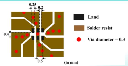
•Line width should be designed to match  $50\Omega$  characteristic impedance, depending on PCB
