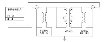
Crosstalk Attenuation — In the dual packages, which contain transmit and receive transformers side by side, sufficient crosstalk attenuation is achieved by the inherent characteristics of the toroid cores as well as by their proper positioning. The crosstalk attenuation is typically 50 dB or better from 100  $\,$  kHz to 10 MHz. This result was established with the test circuit shown below.
