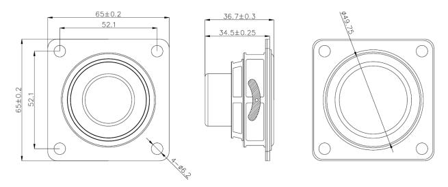
Note: Recommended speaker baffle opening is 53.6mm. Always test-fit prior to closing mechanical design. Please maintain at least 7mm distance between top of frame and next surface.
