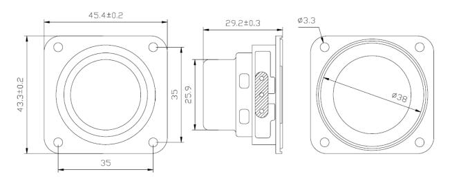
**Note:** Recommended speaker baffle opening is 41mm. Always test-fit prior to closing mechanical design. Please maintain at least 6mm distance between top of frame and next surface.
