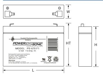
5.95 (151) **W**: 1.34 (34) H: 3.70 (94) HT: 3.94 (100) Tolerances are +/- 0.04 in. (+/- 1mm) and +/- 0.08 in. (+/- 2mm) for height dimensions. All data subject to change without notice.
