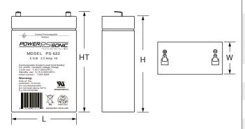
**W**: 1.30 (33) **H**: 4.65 (118) **HT**: 4.80 (122) **L**: 2.60 (66) Tolerances are +/- 0.04 in. (+/- 1mm) and +/- 0.08 in. (+/- 2mm) for height dimensions.
