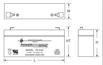
L: 5.28 (134) W: 1.34 (34) H: 2.35 (60) HT: 2.56 (65) Tolerances are +/- 0.04 in. (+/- 1mm) and +/- 0.08 in. (+/- 2mm) for height dimensions. All data subject to change without notice.
