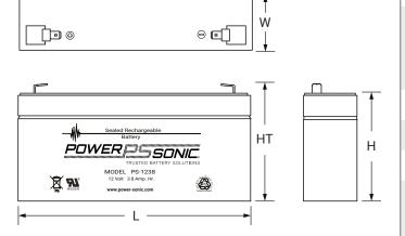
**L**: 7.68 (195) **W**: 1.85 (47) **H:** 2.91 (74) **HT**: 2.99 (76) Tolerances are +/- 0.04 in. (+/- 1mm) and +/- 0.08 in. (+/- 2mm) for height dimensions. All data subject to change without notice.
