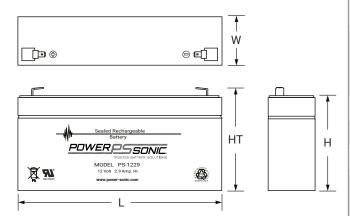
L: 7.00 (178) W: 1.38 (35) H: 2.36 (60) HT: 2.60 (66) Tolerances are +/- 0.04 in. (+/- 1mm) and +/- 0.08 in. (+/- 2mm) for height dimensions. All data subject to change without notice.
