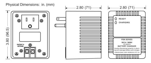
Tolerances are  $\pm$  - 0.04 in. ( $\pm$  - 1mm) and  $\pm$  - 0.08 in. ( $\pm$  - 2mm) for height dimensions.
