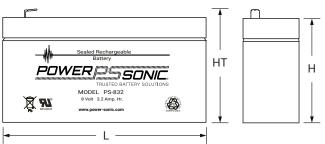
**L:** 5.29 (134) **W:** 1.44 (36.5) **H:** 2.49 (63) Tolerances are  $\pm$  -0.04 in. ( $\pm$ -1mm) and  $\pm$ -0.08 in. ( $\pm$ -2mm) for height dimensions.
