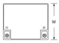
L: 6.54 (166) W: 6.93 (175) H: 4.92 (125) HT: 4.92 (125) Tolerances are +/- 0.04 in. (+/- 1mm) and +/- 0.08 in. (+/- 2mm) for height dimensions. All data subject to change without notice.
