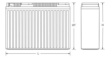
L: 15.50 (394) W: 4.33 (110) H: 11.20 (285) HT: 11.20 (285) Tolerances are +/-0.04 in. (+/-1mm) and +/-0.08 in. (+/-2mm) for height dimensions. All data subject to change without notice.
