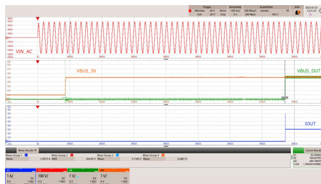
Figure 34 – Input Voltage, Output Voltage and Current. 265 VAC, 5.0 V, 3 A (E-load CC Mode). V_{BUS\_IN} = 5.159 V Steady-State. t_{output\_delay} = 769 ms CH1: IOUT, 1 A / div. CH2: VIN_AC, 100 V / div. CH3: VBUS_OUT, 1 V / div. CH4: VBUS_IN, 1 V / div. Time: 100 ms / div.
