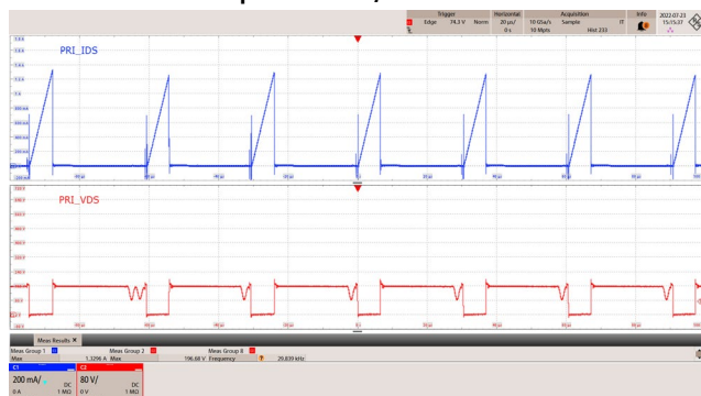
Figure 39 – Primary Drain Voltage and Current. 90 VAC, 5.0 V, 3 A Load. V_{DS\_PRI} = 196.68 V Maximum. CH1: I_{DS\_PRI} , 200 mA / div. CH2: V_{DS\_PRI} , 80 V / div. Time: 20 \mu s / div.
