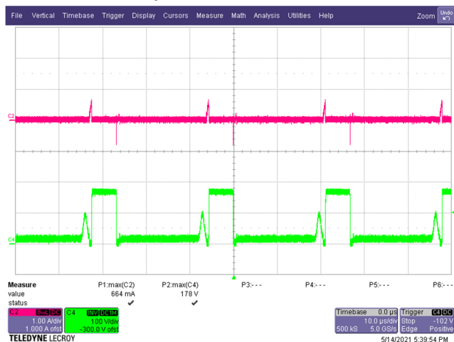
Figure 44 – Primary Clamp Drain Voltage and Current. 90 VAC, 5.0 V, 3 A Load (178 V MAX ). C4: V DRAIN , 100 V / div. C2: I DRAIN , 1 A / div. Time: 10 μs / div.
