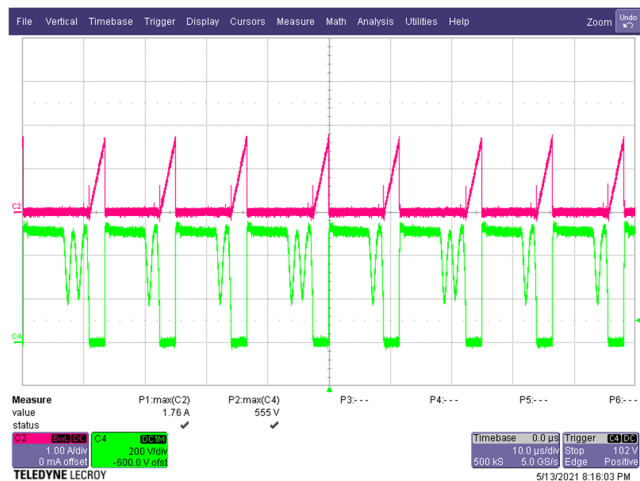
Figure 43 – Primary Drain Voltage and Current. 265 VAC, 20.0 V, 3 A Load (555 V MAX ). C4: V DRAIN , 200 V / div. C2: I DRAIN , 1 A / div. Time: 10 μs / div.
