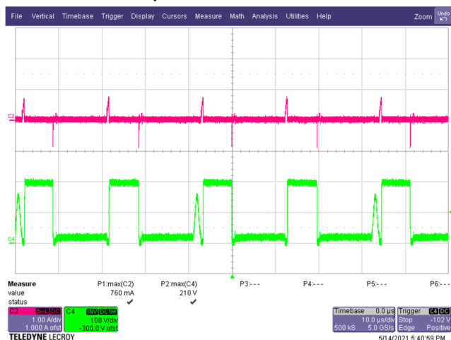
Figure 46 – Primary Clamp Drain Voltage and Current. 90 VAC, 9.0 V, 3 A Load (210 V MAX ). C4: V DRAIN , 100 V / div. C2: I DRAIN , 1 A / div. Time: 10 μs / div.
