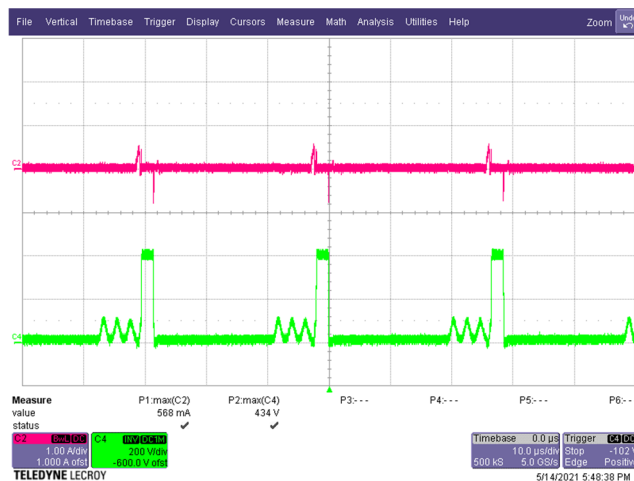
Figure 45 – Primary Clamp Drain Voltage and Current. 265 VAC, 5.0 V, 3 A Load (434 V MAX ). C4: V DRAIN , 200 V / div. C2: I DRAIN , 1 A / div. Time: 10 μs / div.
