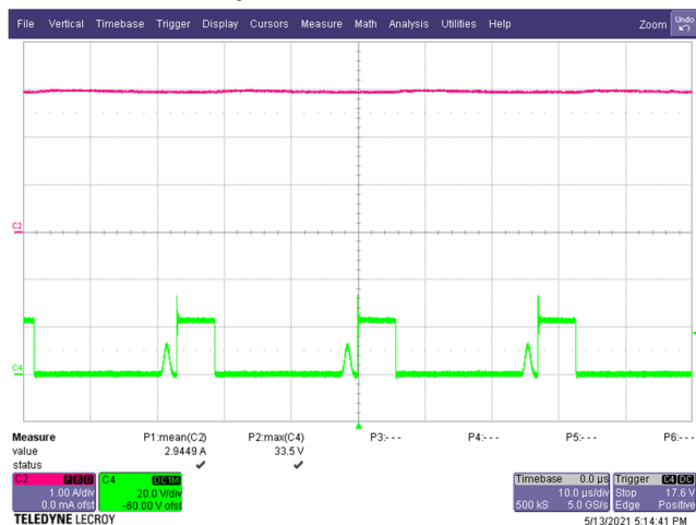
Figure 52 – SR FET Drain Voltage and Current. 90 VAC, 5.0 V, 3 A Load (33.5 V MAX ). C4: V DRAIN(SR) , 20 V / div. C2: I LOAD , 1 A / div. Time: 10 μs / div.
