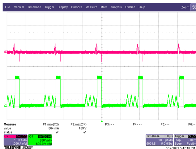
Figure 47 – Primary Clamp Drain Voltage and Current. 265 VAC, 9.0 V, 3 A Load (459 V MAX ). C4: V DRAIN , 200 V / div. C2: I DRAIN , 1 A / div. Time: 10 μs / div.
