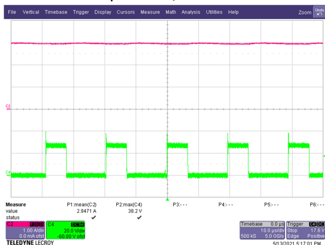
Figure 54 – SR FET Drain Voltage and Current. 90 VAC, 9.0 V, 3 A Load (38.2 V MAX ). C4: V DRAIN(SR) , 20 V / div. C2: I LOAD , 1 A / div. Time: 10 μs / div.
