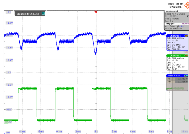
Figure 92 – Transient Output Waveforms. 230 VAC. Upper: V_{OUT} , 400 mV / div., 2 ms / div. Lower: I_{OUT} 200 mA / div. Load Transient: 5 % - 100%. Duty Cycle, Slew Rate: 50%, 0.8 A / \mu s. Frequency: 250 Hz. V_{MAX} : 12.31 V, V_{MIN} : 11.57 V.
