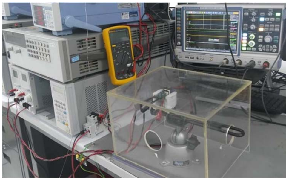
Figure 136 – Thermal Performance Set-up Using an Acrylic Box.
