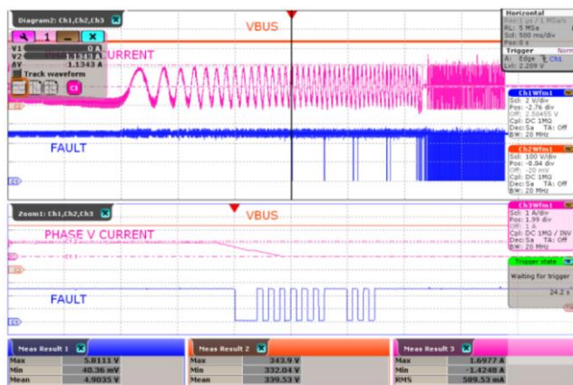
Figure 45 – OCP at R_{XL}/R_{XH} = 115 \text{ k}\Omega , I_{LIM} = 1 \text{ A} .
