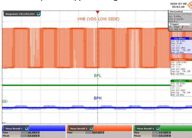
Figure 32 – BPL and BPH Signal at Light Load.
